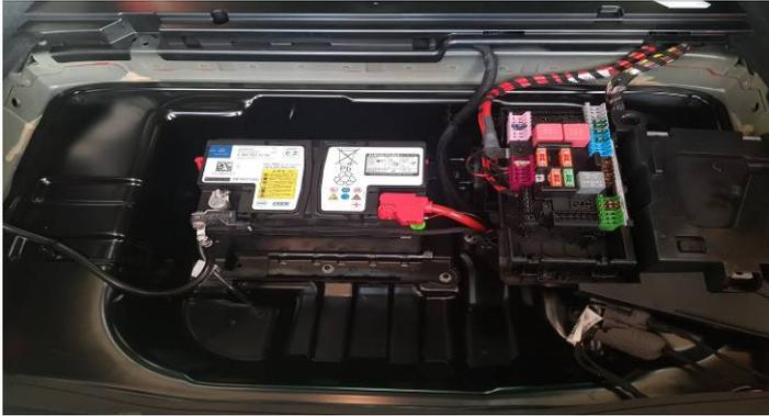
MB moved the ECUs from the trunk, therefore you need to locate the can-bus under the plastic cover in the rear trunk.
