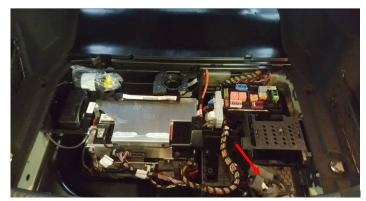
**Step 2)**Locate the 4-pin connector plug of the exhaust valves.
