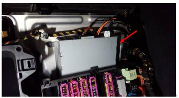
Clip the black carrier out of the housing and remove.
