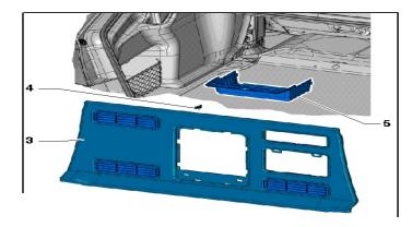
In order to remove the bottom covers, you need to remove the covers of the back seats first.
