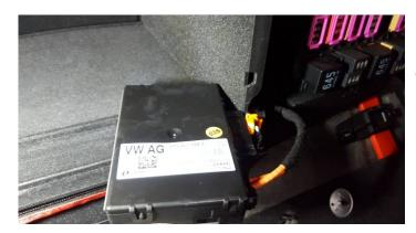
Alternatively, you can also pick up the wire at the CAN gateway.
