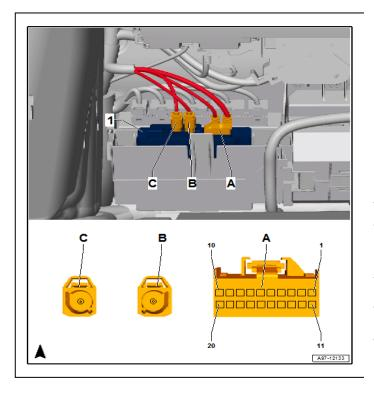
Locate the control unit for the reversing camera.
