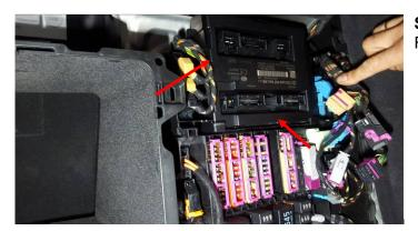
**Step 2)**First, remove all cables to unclip the control module.
