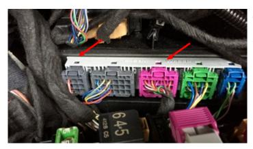
Connect the cables with the adapter.
