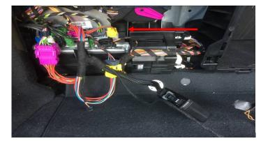
Locate the control module on the left half. It is directly visible.
