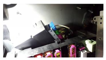
In order to remove the bottom covers, you need to remove the covers of the back seats first.
