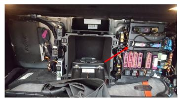
**Step 1)**You will find the control module of the air suspension behind the Comfort control module.
