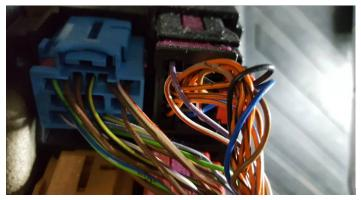
**Step 2)**Unplug the black connector from the socket and insert our Plug/Play Adapter.
