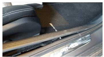
For the Coupé/Cabrio we in any case recommend to lay the Can-Wire to the front right site entry panel and to connect the needed color of chapter 7.1 or 7.2 directly at that place.
