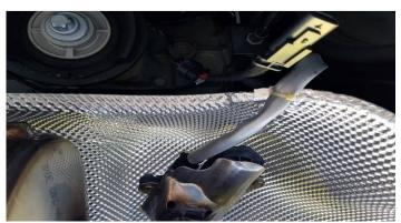
We recommend to lay the wire above the heating protection sheet, to avoid temperature problems.
