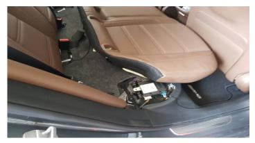
The rear seats are simply clipsed in, when removing the seats, take care about connected plugs.
