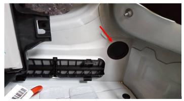
This is an example rubber which can be used for laying the wires to the outsite.
