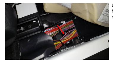
Usually it is enough to lift up the carpenter a bit to find the needed can wires. A full remove is mostly not required.
