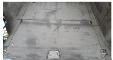
**Step 1)**Open the trunk and remove the coverings to the bottom part of the trunk.
