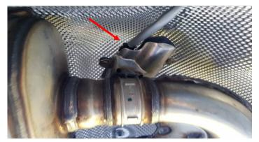
**Step 2)**Remove the plug from the exhaust valve motor.
